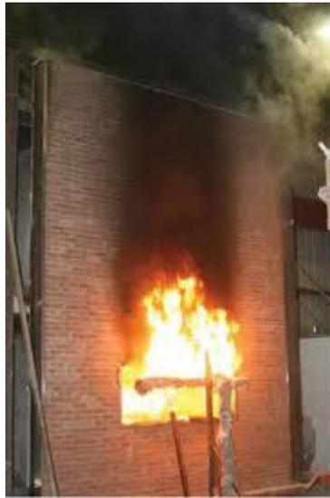
Figure 1: NFPA 285 test in progress.
